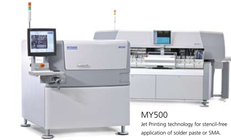
MY100LXe-10/14 All-in-one mounter. Featuring up to 176 feeder positions with a top speed of 16,000 components per hour. Upgradeable to MY100SXe.
